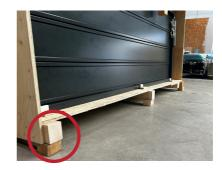
Prior to opening the crate, blocks should be used to lift the base of the crate. The crate must be inclined to the rear at an angle of ca. 5°. This prevents the windows from falling out when the transport lock is released. This prevents the windows from falling out when the transport lock is released.
